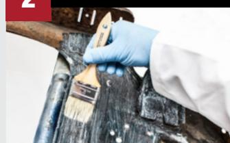
Apply 2 – 3 light coats of **Rust Seal** 5 – 10 minutes apart. Do not apply to sand blasted or painted areas. Allow to dry fully. **Rust Seal** does not require a top coat unless exposed to outdoor conditions. Body filler and top coat can be used after **Rust Seal** has fully dried.
