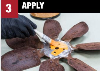
Apply 2 – 3 medium wet coats of **Rust Shield** with a brush or spray gun allowing a 3 – 5 minute flash time between coats. Maximum rust protection is achieved from thicker applications. Allow final coat to cure 24 – 48 hours before returning part to service.
