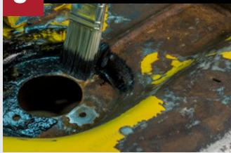
Apply 2 medium coats of **Rust Trap** with a brush or spray gun. First coat should not achieve full coverage and second coat should be applied in the same manner while first coat is still wet. Allow final coat to cure for 8 – 24 hours before returning part to service.
