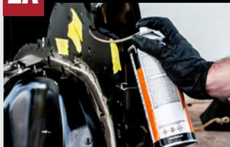
Clean surface with **SEM Solve** or **XXX Universal Surface Cleaner** where applicable. Remove cap from **Rust Preventer Cavity Wax**, attach straw or **Rust Preventer Aero Wand**. Apply 1 – 2 coats.
