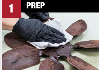
Remove loose scale with a wire brush. Clean with **SEM Solve** to remove oil, grease and dirt. Blow off with compressed air.
