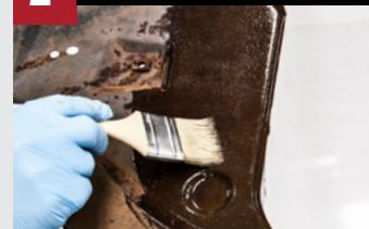
Dip smaller parts or brush onto larger parts. When applying **Rust Mort** by brush, keep product wet throughout the conversion process.
