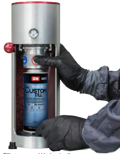
Filling an aerosol blank using the Custom Fill Pneumatic Machine
